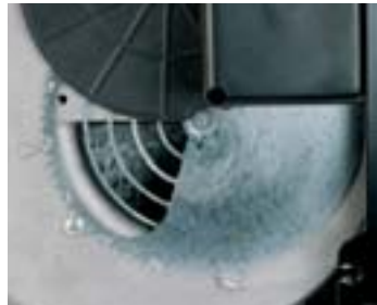
Air damper partially open (GS10, GS20)
