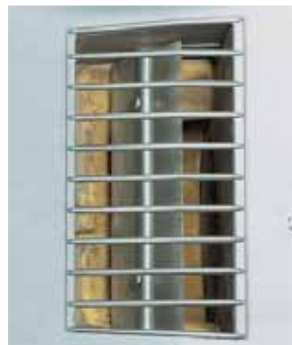
Example of the air damper on RL 50 burners.
